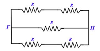
The equivalent resistance between F and H is the resultant of resistances, 2R, R and 2R connected in parallel. Therefore,
