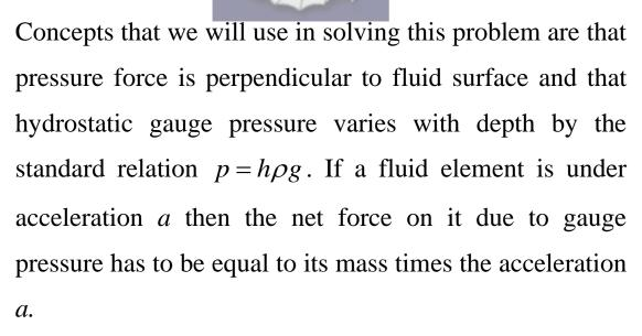
We consider an element of the fluid that is moving horizontally with acceleration. Relevant data concerning the motion of this element have been shown in the
